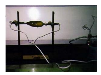
6. At first, the pickle will start dripping. Then it will start to hiss and smoke and then it will really start glowing. And it will smell!!! Make sure you unplug the unit before removing the pickle.
